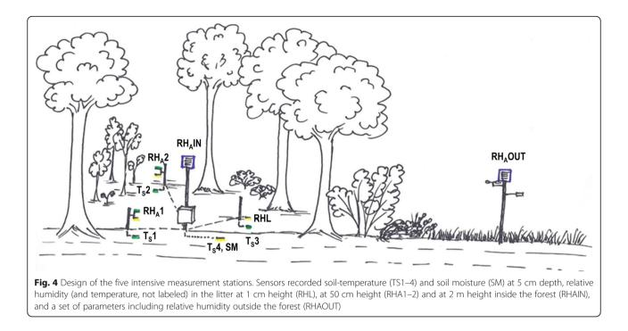
shield and fastened at 50 cm height on a wooden post (Fig. 3). For a high comparability of conditions measured at 50 cm height over all study sites, the post was located as far as possible from any trees or shrubs.
