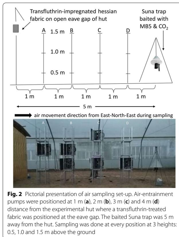
**Fig. 2** Pictorial presentation of air sampling set-up. Air-entrainment pumps were positioned at 1 m (a), 2 m (b), 3 m (c) and 4 m (d) distance from the experimental hut where a transfluthrin-treated fabric was positioned at the eave gap. The baited Suna trap was 5 m away from the hut. Sampling was done at every position at 3 heights: 0.5, 1.0 and 1.5 m above the ground
