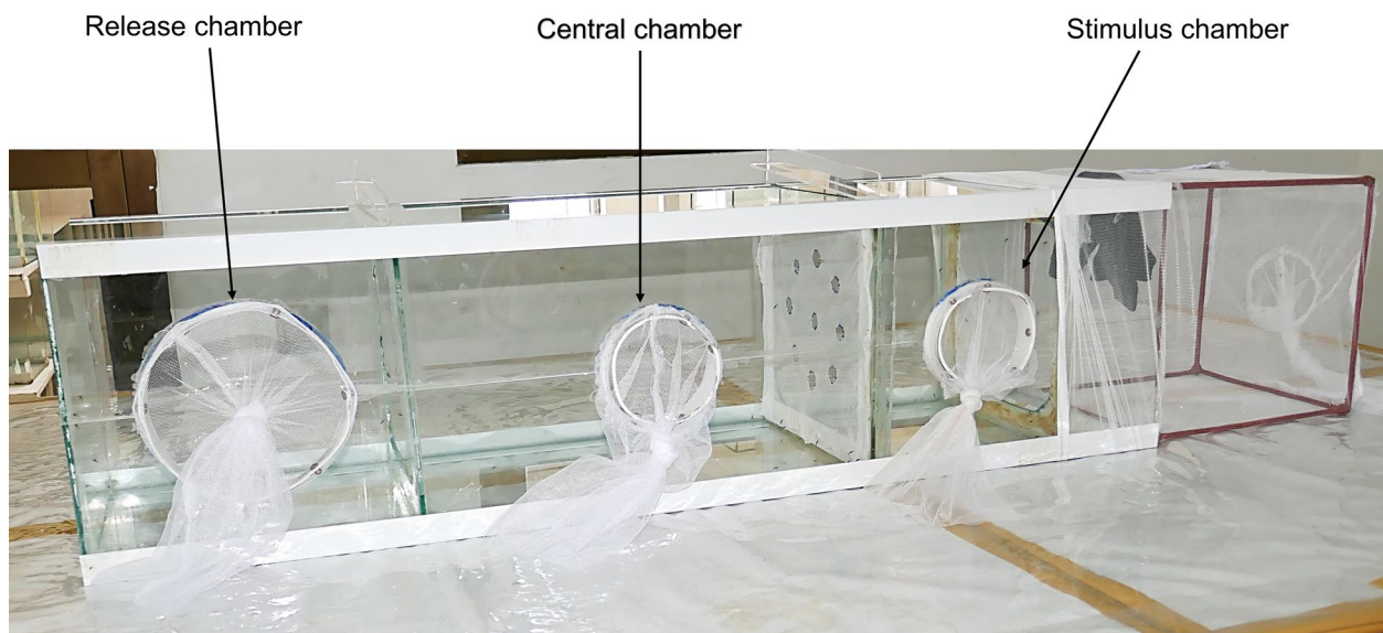
Fig. 1 Modified WHO tunnel assay. The main sections are the release, central and stimulus chambers. The partition between the central chamber and the response chamber was designed to attach individual test-treated nets or control. To protect mosquitoes from escaping, the extension cage was made from a Safi net with 100 deniers that do not allow the mosquito to pass and socks placed in the stimulus chamber as a bait to lure mosquitoes towards the test-treated nets or control
