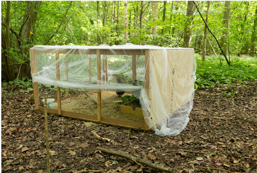
Fig. 1 Chicken baited trap with lifted mosquito net
