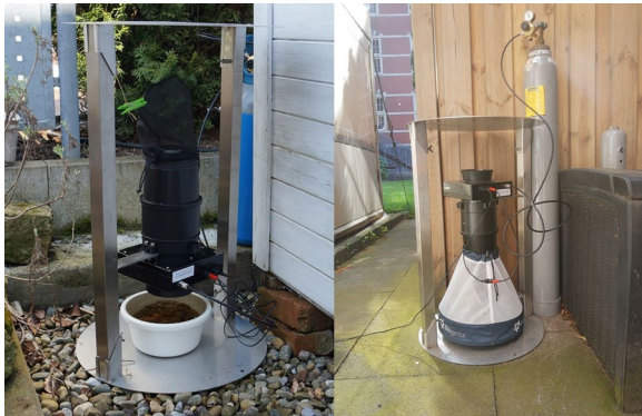
Fig. 1 Trap versions: CO 2 -Pro-gravid (left) and CO 2 -Pro (right), each equipped with a BG-Counter 2 in combination with the BG-Pro and BG-Trap-Station
