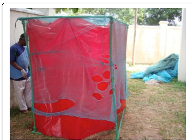
Figure 2 Damaged LLINs being examined on a plastic frame showing distribution of large holes (>5 cm) and knots as a method of net repair.
