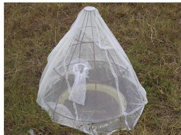
Figure 1 Standardized field test set up. Netting-covered emergence trap on top of artificial pond.
