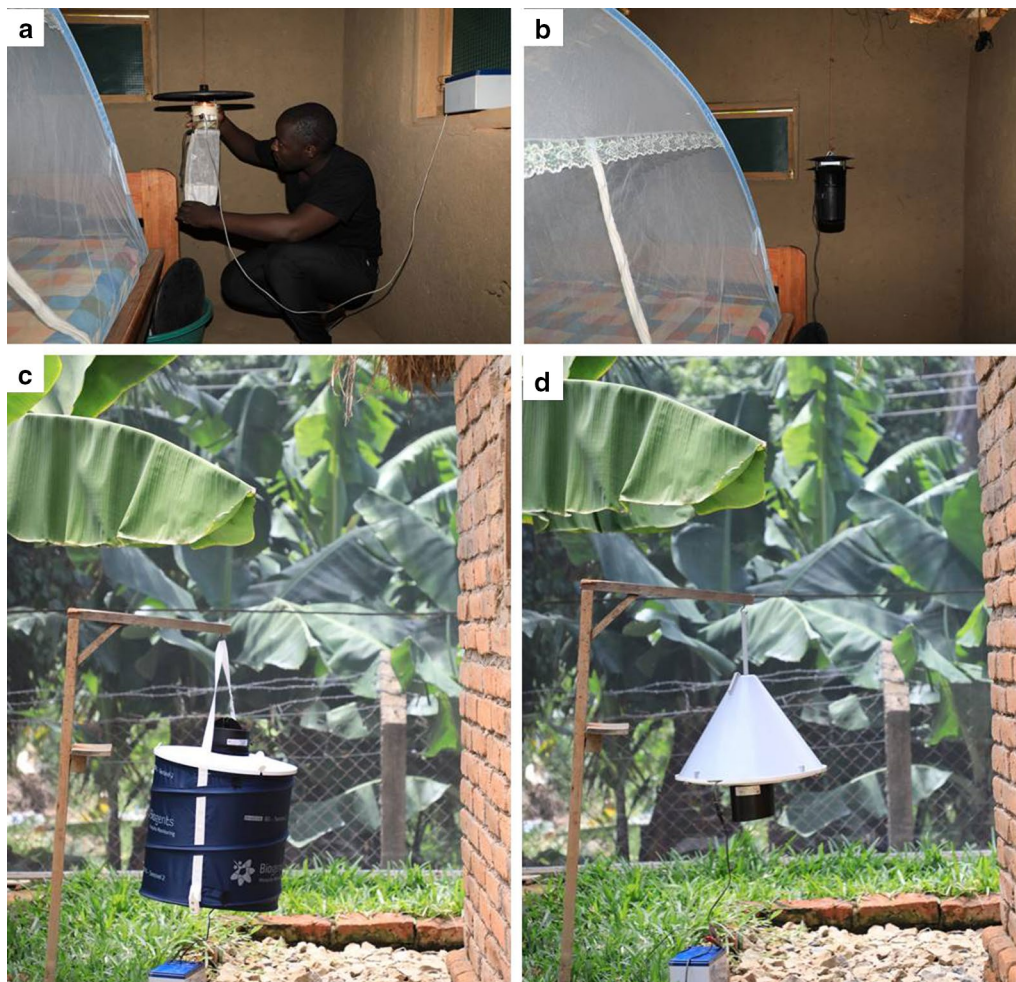
Fig. 3 Images of trap set up during semi-field experiment, a CDC-Light trap set up indoors beside a bed with a bednet. b Mosclean trap indoors beside a bed with a bednet. c BG-Sentinel trap set up outdoors. d Suna Trap set up outdoors
