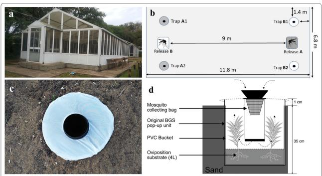
**Fig. 2** Overview of experimental set-up in the large field cages (**a**) with schematic overview of mosquito release points and trap positions (**b**). The white and blue colours show the trap locations and their respective mosquito release points. Test substrates were provided in modified BG-Sentinel traps buried in the ground (**c**). The cross-section through the modified BG-Sentinel gravid trap (**d**) shows the location of the plants and the airflow generated by the trap
